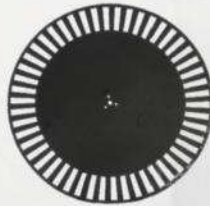
JOHN LOGIE BAIRD'S SCANNING DISCS - THE EARLIEST EXPERIMENTS IN TELEVISION (1924-28)
